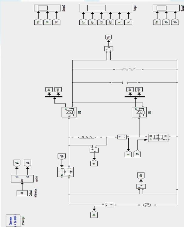
**Figure 7: Simulation model of bridgeless boost rectifier**
