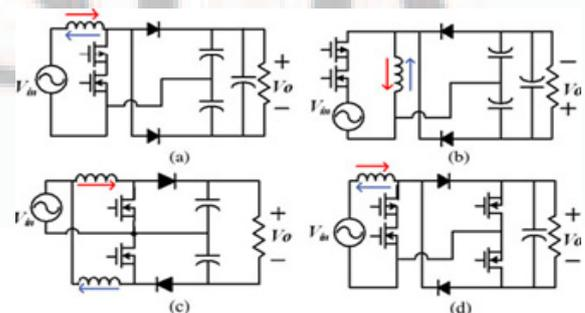
**Figure 2:** Bridgeless ac-dc converters [6]. (a) Split capacitor boost converter. (b) Split capacitor buck-boost converter. (c) Dual polarity boost converter. (d) Boost converter with secondary switches.
