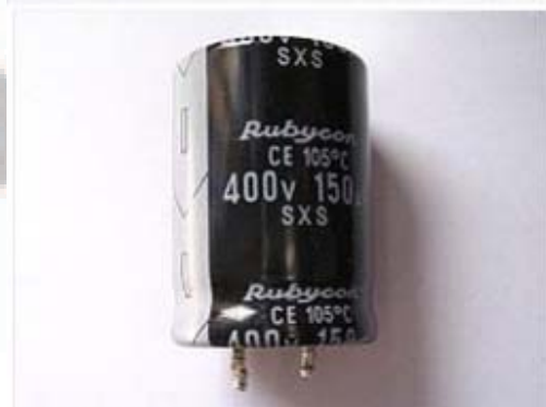
A typical electrolytic capacitor
