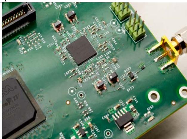
Figure 8: Wideband RF Transceiver
