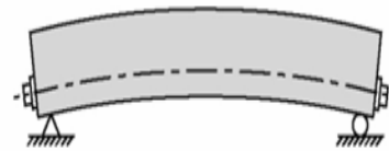
b. Post-tensioned concrete before loading
