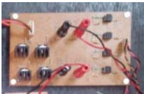
Figure 3: Connections of MOSFETs with battery and motor
