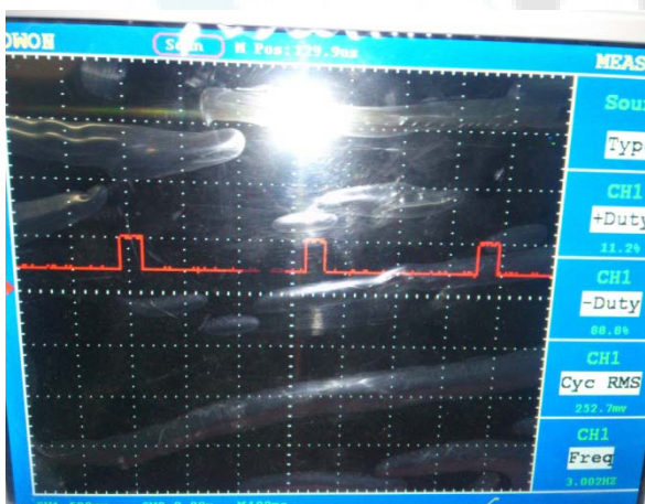
Figure 5: Waveform achieved at zero accelerator
