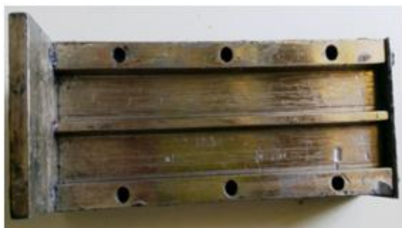
Figure 2: Metallic Die for specimen preparation
