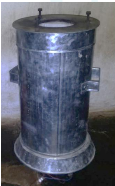
Figure 1: Fabricated cook stove
