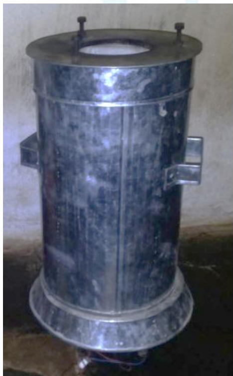
Figure 1: Fabricated cook stove
