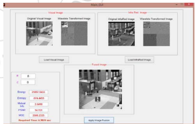
Figure 4: Fusion result for visual and IR image
