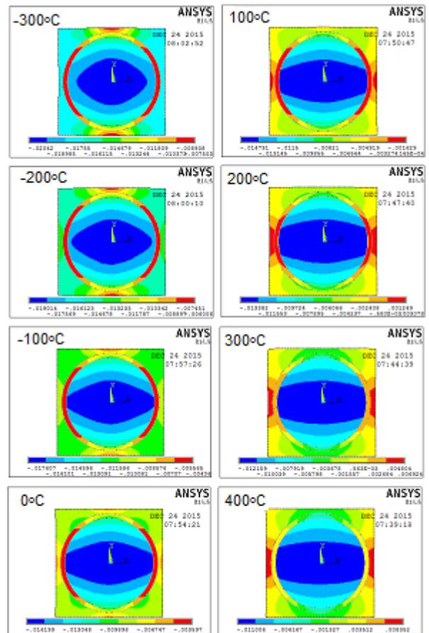
Figure 5: Raster images of thermo-elastic strain of AA7020/30% TiC composites.
