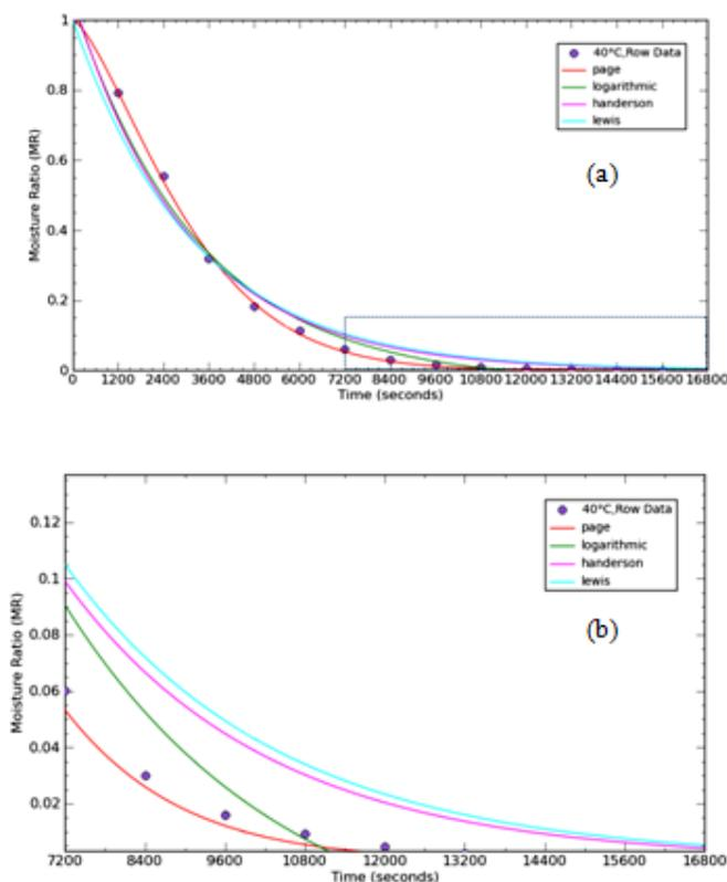
**Figure 2:** Values of moisture ratio in 40 °C fitted with four thin-layer drying models (a). Dotted line sector in figure (2-a) is magnitude in figure (2-b).
