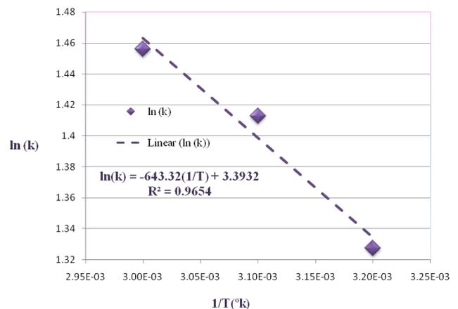
**Figure 3:** Arrhenius curve of total weight to solid weigh ratio (k) data at 40, 50 and 60 °C. Dotted line shows average values of total weight to solid weigh ratio in each experimental temperature.
