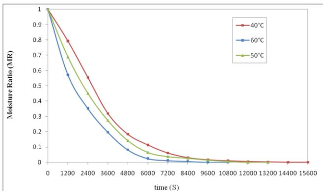
**Figure 1:** Drying curves for cucumber slices at three different temperatures
