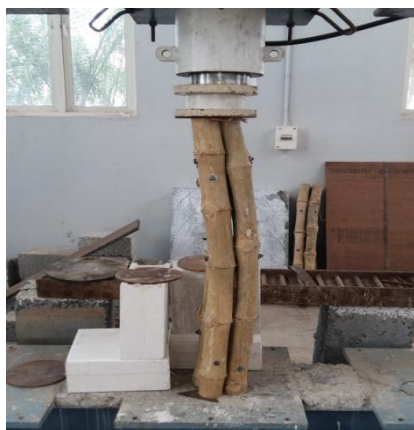
Figure 12: Bending pattern of column
