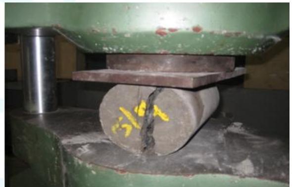
Figure 3: Split Tensile Strength on cylinder
