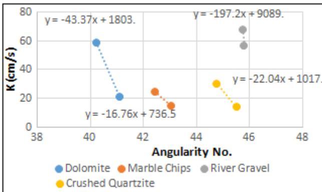
**Figure 7:** Angularity vs Hydraulic Conductivity
