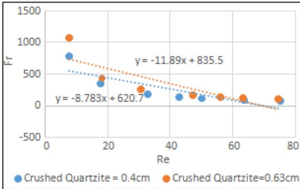
Figure 5: Fr-Re Curve for Crushed Quartzite
