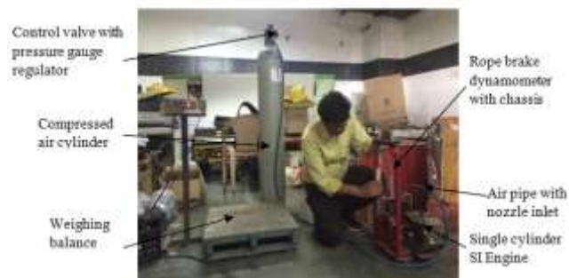
Figure 3: Experimental set up for 4 stroke single cylinder air engine
