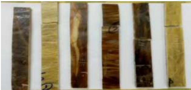
Figure 3: Tensile test Specimens
