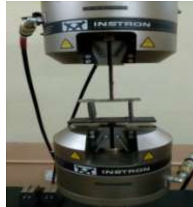
Figure 4: Sample loaded in Instron 8801
