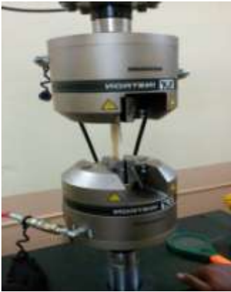
Figure 2: Sample loaded on Instron 8801
