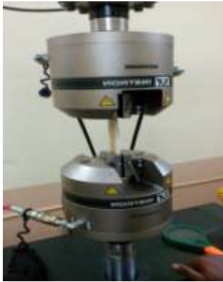
Figure 2: Sample loaded on Instron 8801
