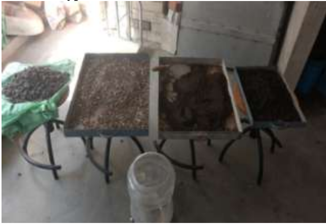
Figure 17: Materials used in slow sand filter
