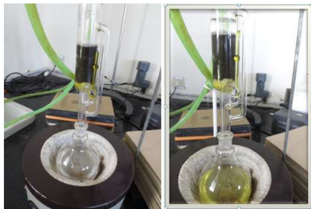
Figure 2: Soxhlet extraction of biofuel from oscillatoria
