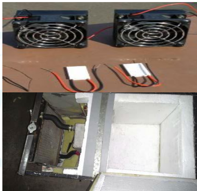
Figure 2: Schematic Diagram of developed thermoelectric refrigeration cabinet
