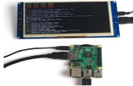
Figure 7: Touch LCD Display connected to Raspberry pi
