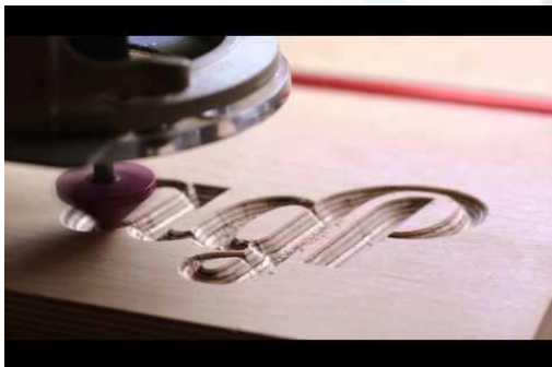
Figure 3: Letters being etched by a CNC header
