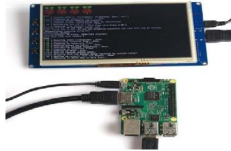
Figure 7: Touch LCD Display connected to Raspberry pi
