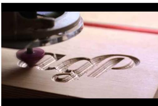
Figure 3: Letters being etched by a CNC header
