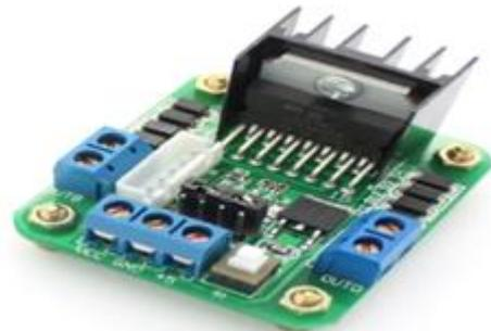
Figure 4: Stepper motor driver board
