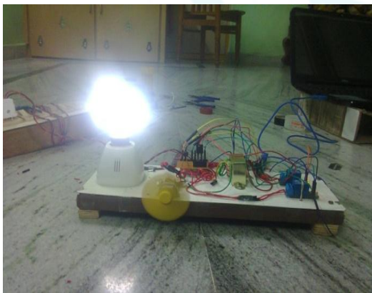
Figure 21: Both load 2(i.e. bulb) and load 1 (i.e. fan) are in on position
