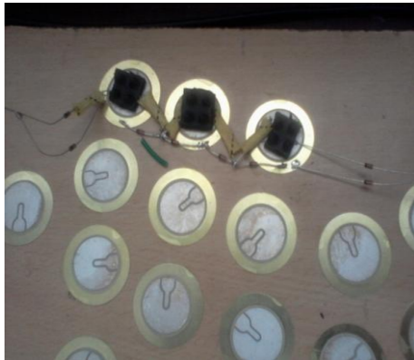
Figure 3: PZT in series connection
