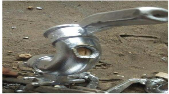
Figure 6: Defective casting part
