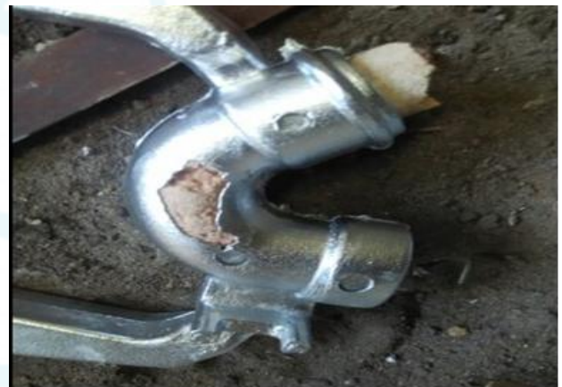
Figure 8: Defective casting part
