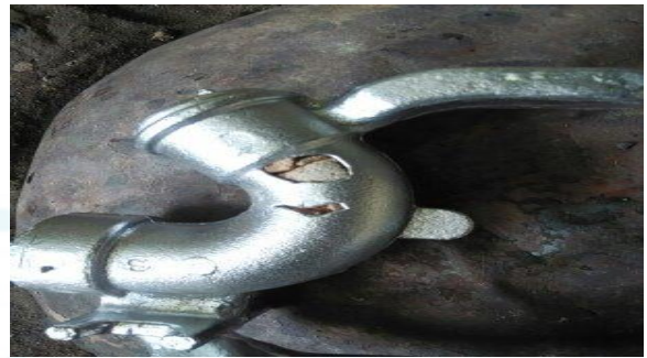
Figure 7: Defective casting part
