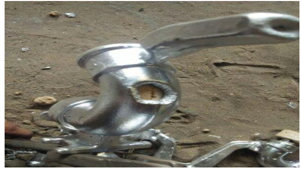
Figure 6: Defective casting part
