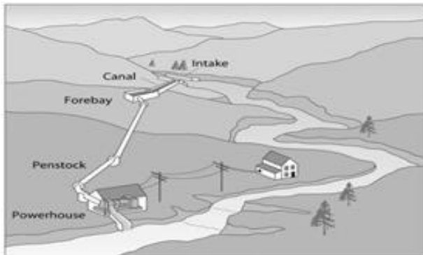
Figure 1: Layout of a Hydropower plant (From: Microhydro-power systems. [Online]. ENERGY.GOV, 2012. [Viewed 31/05/2015]. Available from: http://energy.gov/energysaver/articles/microhydropower-systems )
