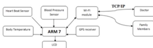
The key components in this block diagram are ARM 7 microcontroller, Heart Beat/BP sensor, Body Temperature sensor, GPS Receiver, Wi-Fi Module and LCD.
