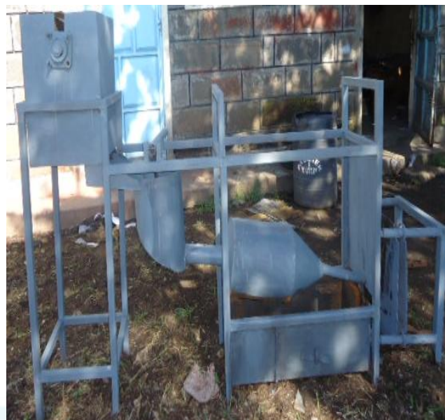
Figure 6: Fabricated injection moulding machine
