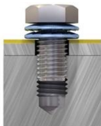
Figure 2: Tapped hole showing thread engagement
