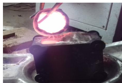
Figure 1: Molten material at pouring condition
