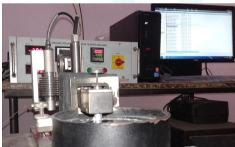
Figure 3: Pin on disc apparatus set up
