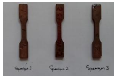
Figure 5: Standard samples for tensile test
