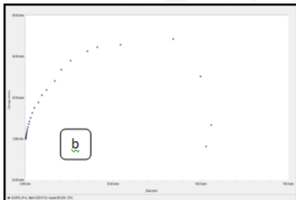
Figure 9: Effect of Nyquist curve for aluminum (a) in 0.025M TCA and (b) 0.025M TCA in presences of 12 ml TC extract
