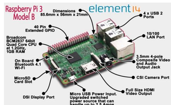
The Pin Headers provide a massive **amount of connectivity**, making raspberry pi a suitable platform for product development for physical computing and “internet of things” devices.
