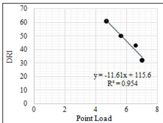
Figure 3.5: Plot of DRI against Point Load
