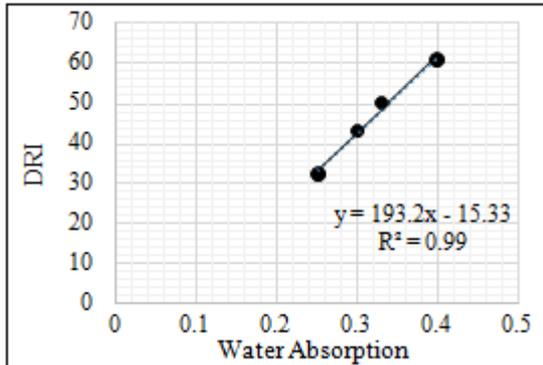
Figure 3.3: Plot of DRI against Water Absorption
