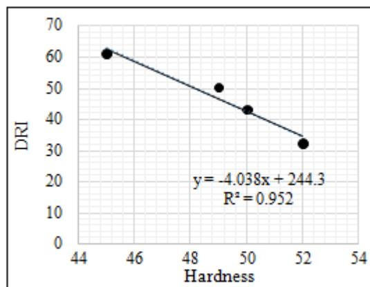
**Figure 3.1:** Plot of DRI against Hardness
