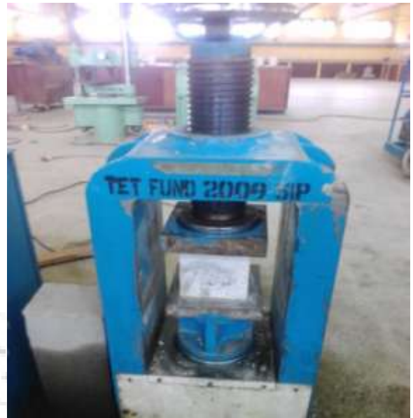
Plate 1: Compressive strength test setup
