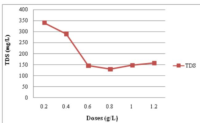
**Fig 3.3:** Effect of Coagulant dosage on TD
