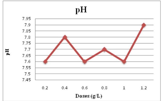
Fig 3.5: Effect of coagulant dosage on pH
