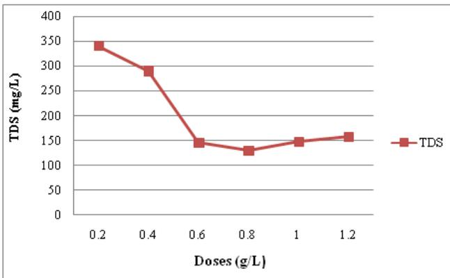
Fig 3.3: Effect of Coagulant dosage on TD
