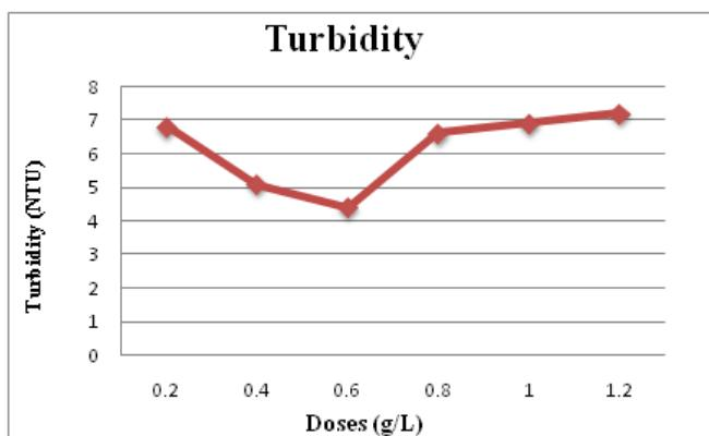
**Fig 3.2:** Effect of Coagulant dosage on Turbidity
