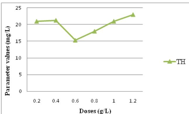
Fig 3.4: Effect of Coagulant dosage on Total Hardness
