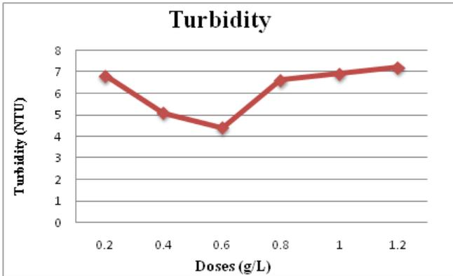
Fig 3.2: Effect of Coagulant dosage on Turbidity
