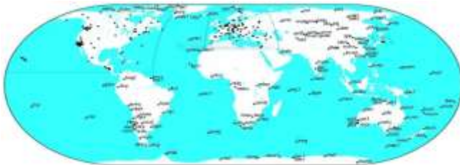
Figure 1: IGS directly manages ~400 permanent GNSS stations observing 4-12 satellites at 30 s rate: more than 250,000 STEC observations/hour worldwide, but there is lack of stations at some areas (e.g., over the oceans).
