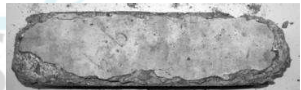
Figure 15: Specimens 28 th day immersion in a 4% concentrated Chloride solutions under freeze and thaw conditions
