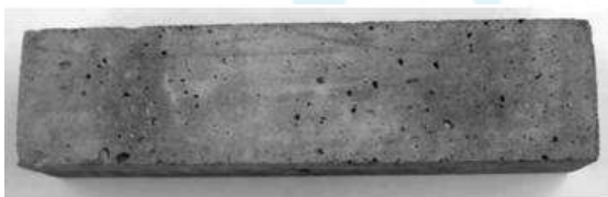
Figure 19: Specimens with 7% air masses later in 14 days of dipping in 6% concentrated solution.
