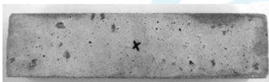
Figure 18: Specimens with 2% air masses after 14 days of dipping within the concentrated solution
