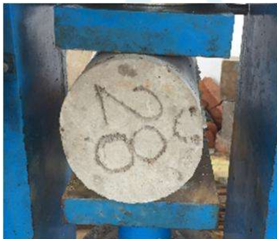
Figure 4: Cylinder placed in CTM
