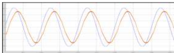
Figure 20: Simulation results of the proposed topology with leading power factor operation. (a) vg [500 V/div] and (b) ig [2 A/div]
