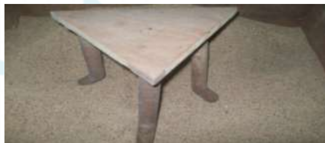
Figure 1: Group of three pile model on which experiments was don
