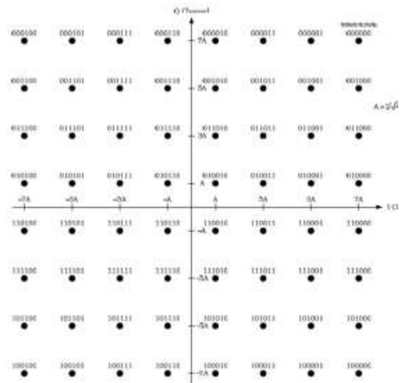
Figure 3: Constellation diagram of 64 QAM
