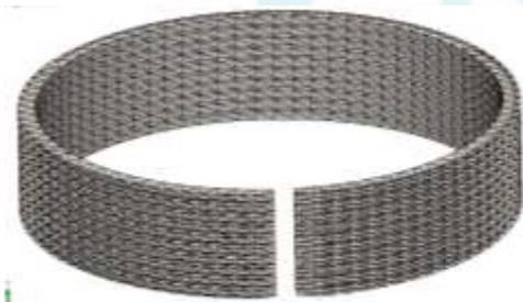
Figure 6: Meshed Model of I-Section Rings
