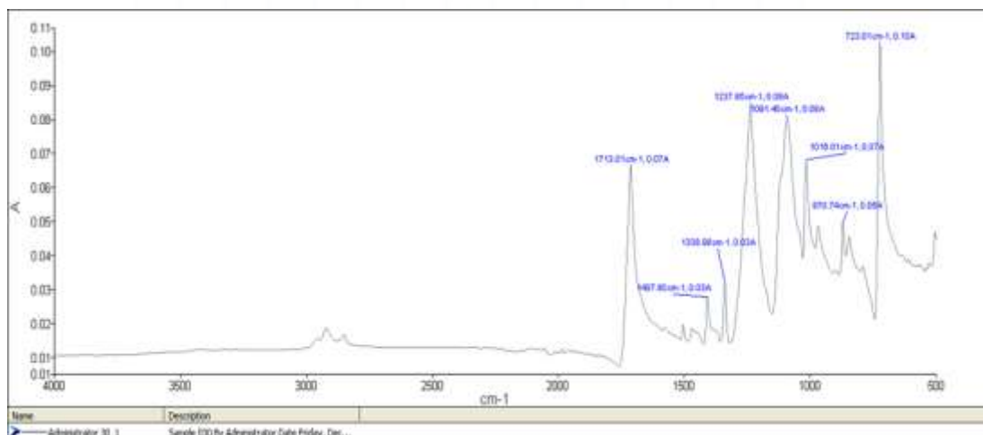
Figure 4: FTIR result of untreated polyester fabric
