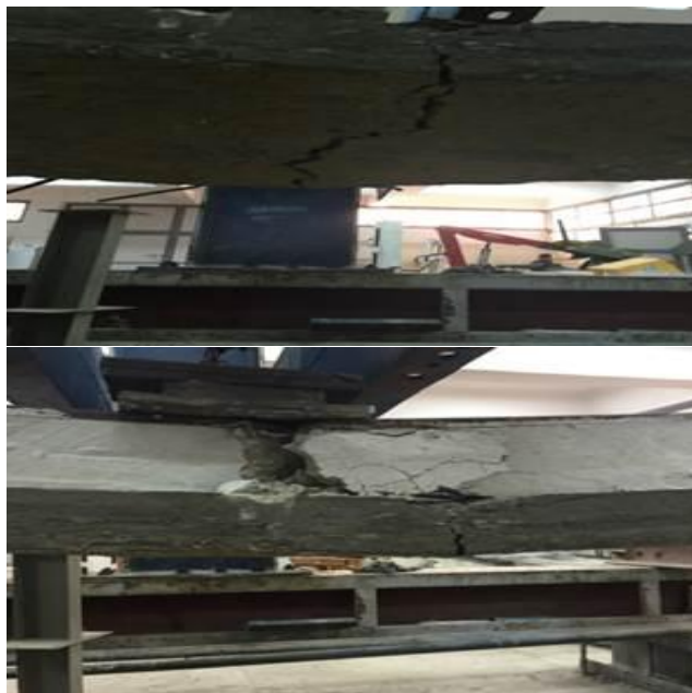
Figure 5.d: Cracks in the concrete slab followed by plastic hinge appeared in the mid span (A-5)
