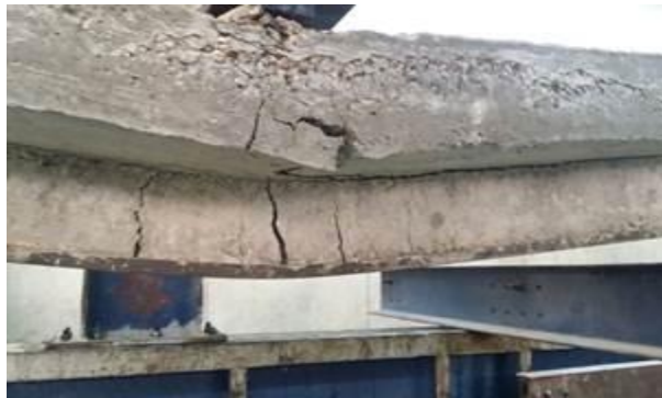
Figure 5.c: Web encasement effect (A-6)
