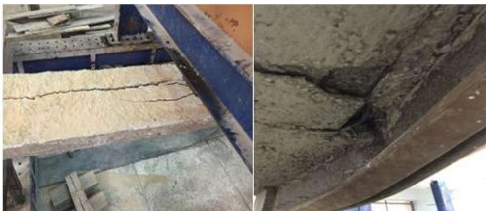
Figure 5.a: Longitudinal cracks in the concrete slab beam followed by flexural buckling of the upper flange and web of steel section in the mid span (A-2)
