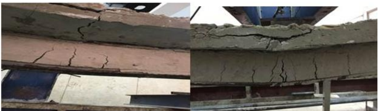
Figure 6: Concrete cracks in the mid span (B-2)
