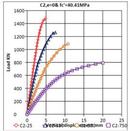
**Figure 10:** The Load-Vertical Displacement Curve for Column Specimens of Group one series C2
