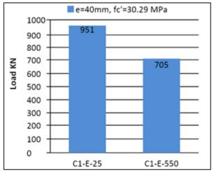
**Figure 11:** Ultimate Axial Load of SRC Columns For Group two series C1
