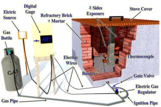
Figure 3: burning process and stove details
