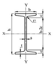
Figure 1: Sectional Properties of I-Section
