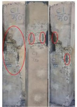
**Figure 18:** failure mode of (Specimen C1-750) crushing of concrete and local buckling for steel
