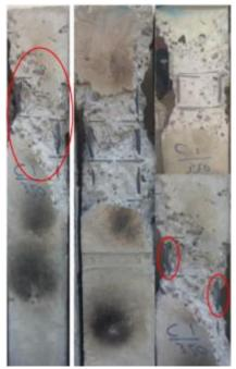
**Figure 16:** failure mode of (Specimen C1-350) crushing of concrete and local bucking for steel
