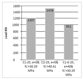
**Figure 5:** Ultimate Axial Load of SRC Columns at Room Temperature
