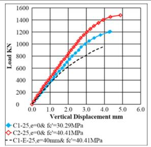
Figure 6: the load-vertical displacement curve for SRC columns at room temperature
