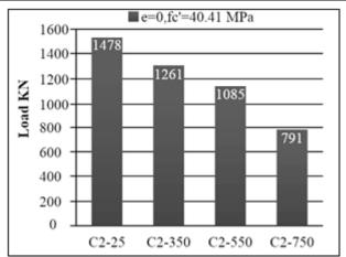
**Figure 9:** Ultimate Axial Load of SRC Columns For Group one series C2
