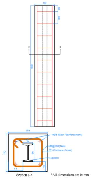
Figure 2: Details of SRC Column Specimens
