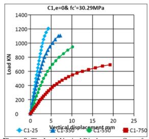
**Figure 8:** The Load-Vertical Displacement Curve for column Specimens of Group one series C1
