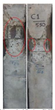
**Figure 17:** failure mode of (Specimen C1-550) crushing of concrete and local buckling for steel
