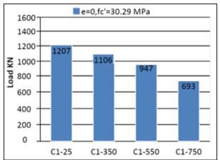
Figure 7: Ultimate Axial Load of For Group one series C1
