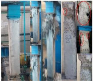
**Figure 14:** failure mode of (Specimen C2-25) ) crushing of concrete and local buckling of steel
