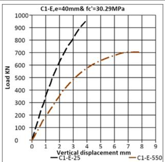
**Figure 12:** the Load Vertical-Displacement Curve for Column Specimens of
