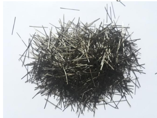
Basalt fibre 24 mm in length
