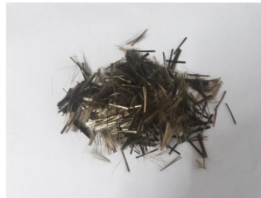
Basalt fibre 18 mm in length
