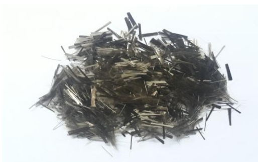
Basal Fibre 12 mm in length
