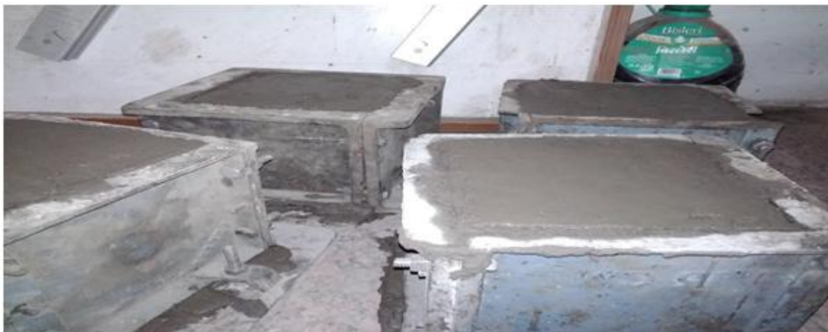
Figure 3.9: Casting of cubes
