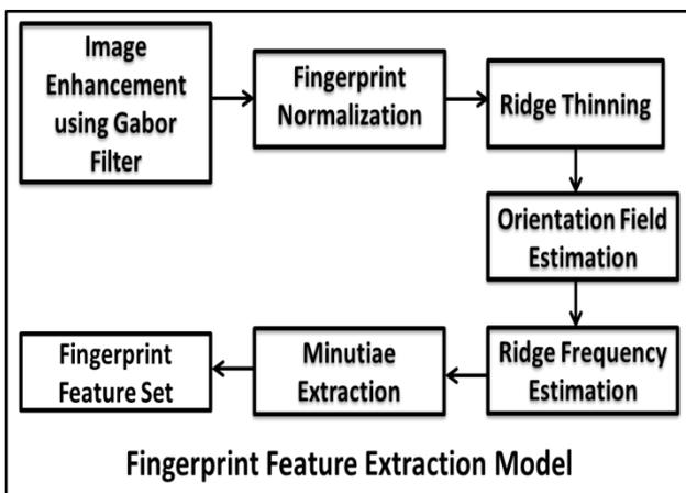
Figure 5. Fingerprint Feature Extraction Model.
