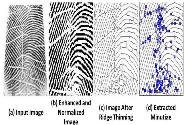
**Figure 6.** Main Steps for Extracting Minutiae from a Fingerprint Image Collected from CASIA Fingerprint Image Database Version 5.0
