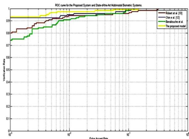
**Figure 9.** The ROC curve for the performance of the proposed system and a number of the state-of-the-art multimodal biometrics systems. The verification rate is plotted at different values of false acceptance rate (1%, 0.1%, 0.01%, 0.001%).
