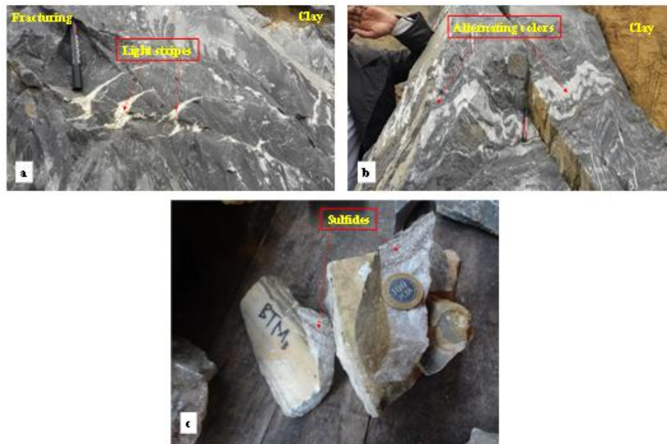
Figure 2: Samples of Doussiegoussou marble northwest of Tchibanga showing fractures and light bands (a), alternating coloring (b) and sulphides (c)
