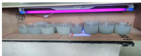
Samples kept under UV box for UV light exposure
