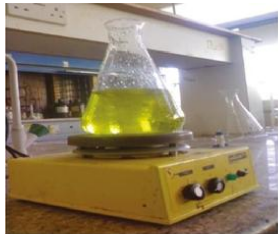
Figure 1: Shows solving of catalyst mixture in oil (60°C)
