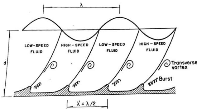
**Figure 5.1:** Alternation of low-speed and high speed fluid bodies and burst-inducing mechanism.
