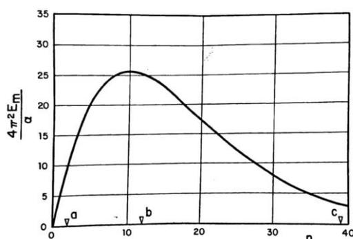
**Figure 7.1:** Energy Spectrum as a function of the frequency number n. Typical experimental values of n are shown for (a) Prandtl eddies, (b) energy-containing eddies and (c) energy-dissipating eddies.
