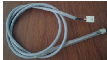
Figure 2: DS18B20 Temperature Sensor with Liquid Isolation.
